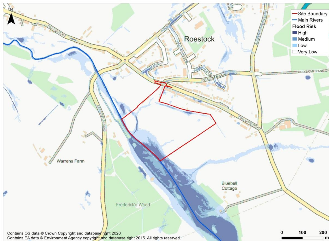
Figure 5-3: EA Risk of Flooding from Surface Water Map
