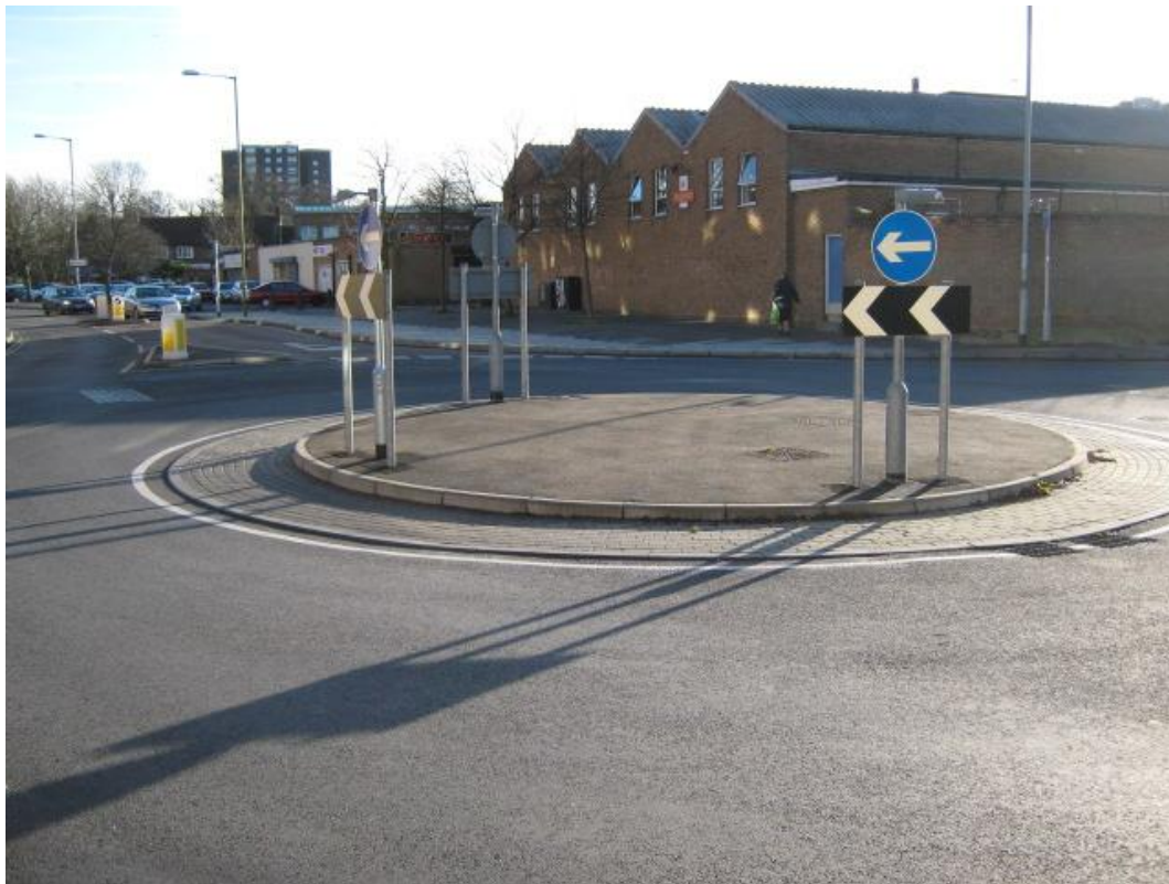
Photo 4.2.1.2: Example of a compact roundabout
