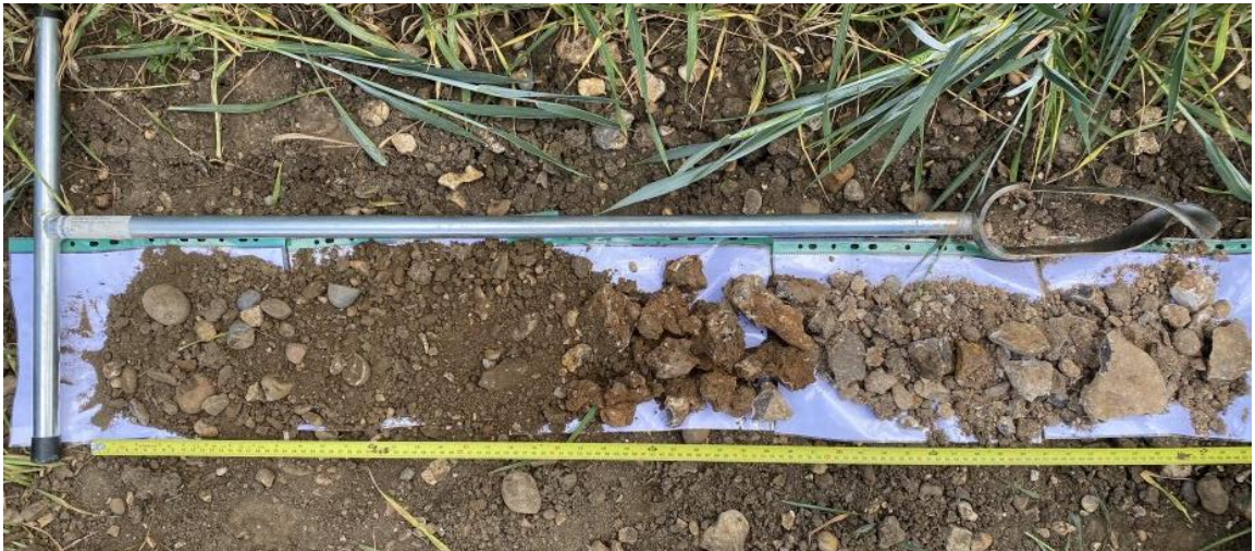
Image 3 – Boring 3 showing a very stony silty clay loam soil in the top horizon, extending to a very flinty and gravelly silty clay loam subsoil. Soil profile is approximately 100cm deep
