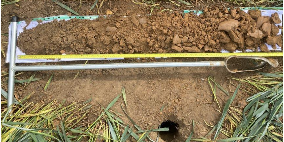
Image 2 – Boring 1 showing a stony silty clay loam, extending to a freely draining silty clay loam soils subsoil, extending to 120cm
