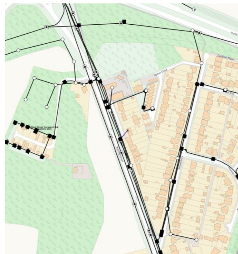
Figure 11 - Existing Openreach infrastructure
