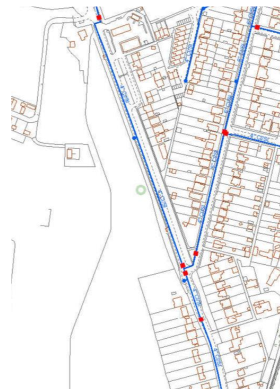
Figure 9 – Existing water apparatus for the northern aspect of the site – Affinity Water asset record
