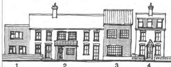
FIG B POOR EXTENSIONS
