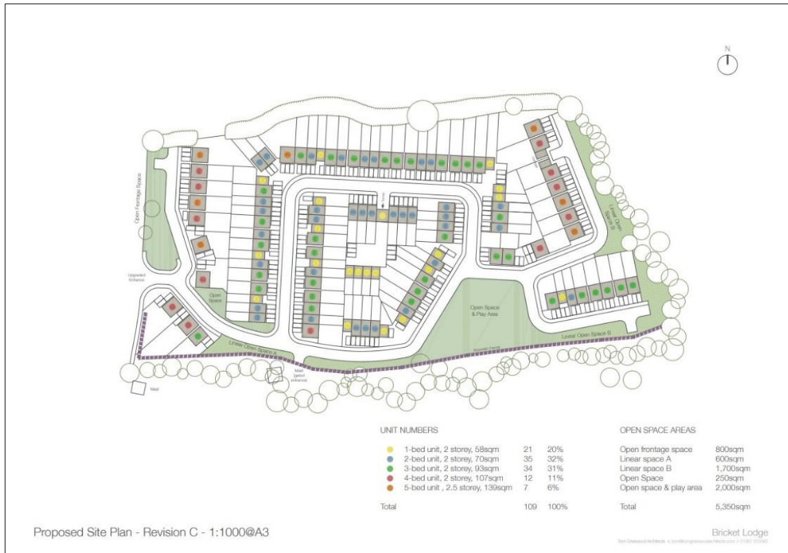
Fig. 3 Indicative Proposed Site Layout, Rev. C (CD 1.4)
