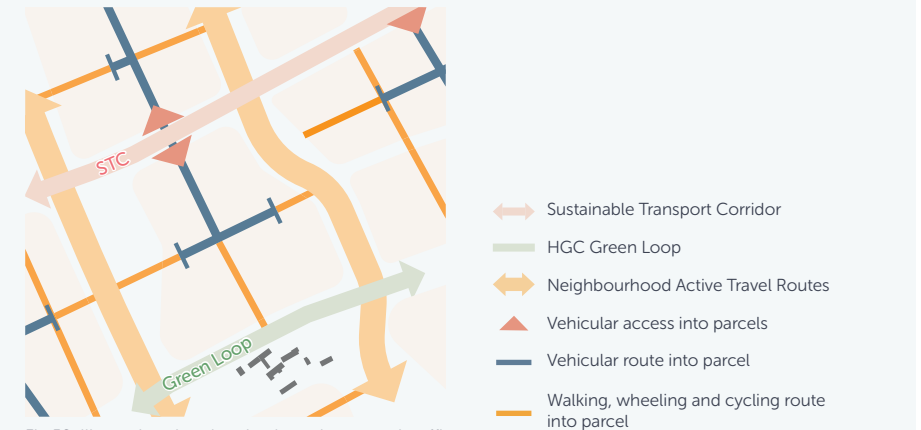
Fig.52 Illustrative plan showing how the general traffic routes, and active travel links can work together to create a walkable, connected network of streets and paths
