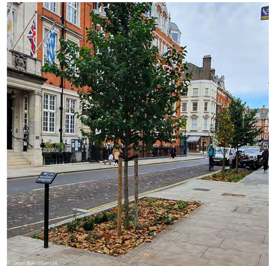
© Green Blue Urban Ltd. Street trees with adequate size tree pit to encourage growth
