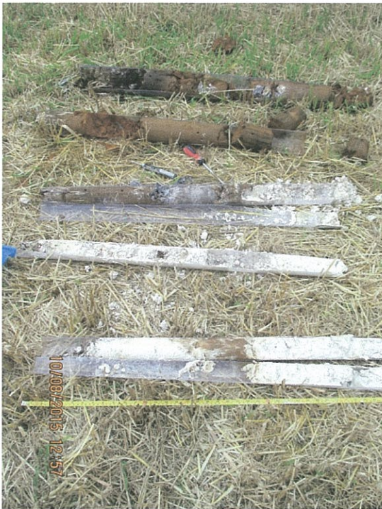
Photo 5: view of the arisings from WS1, showing the boundary between Clay-with-Flints and the underlying Chalk.
