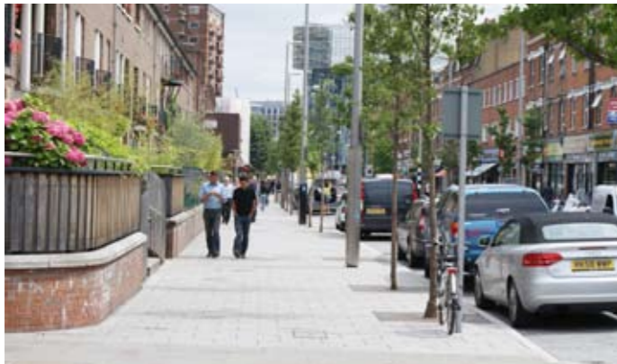
A well defined zone for all street furniture keeps the remaining, 'effective' footway width to a maximum
