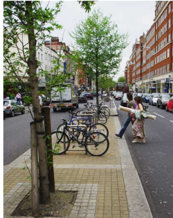
Central medians can be used for additional tree planting, lighting, cycle parking and other street furniture as well as aid crossing
