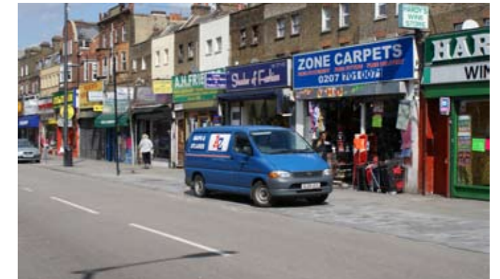
Loading bays at footway level can be utilised by pedestrians as additional footway when not in use
