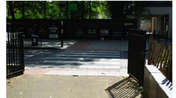
Crossing points should be placed as close as possible to pedestrian desire lines
