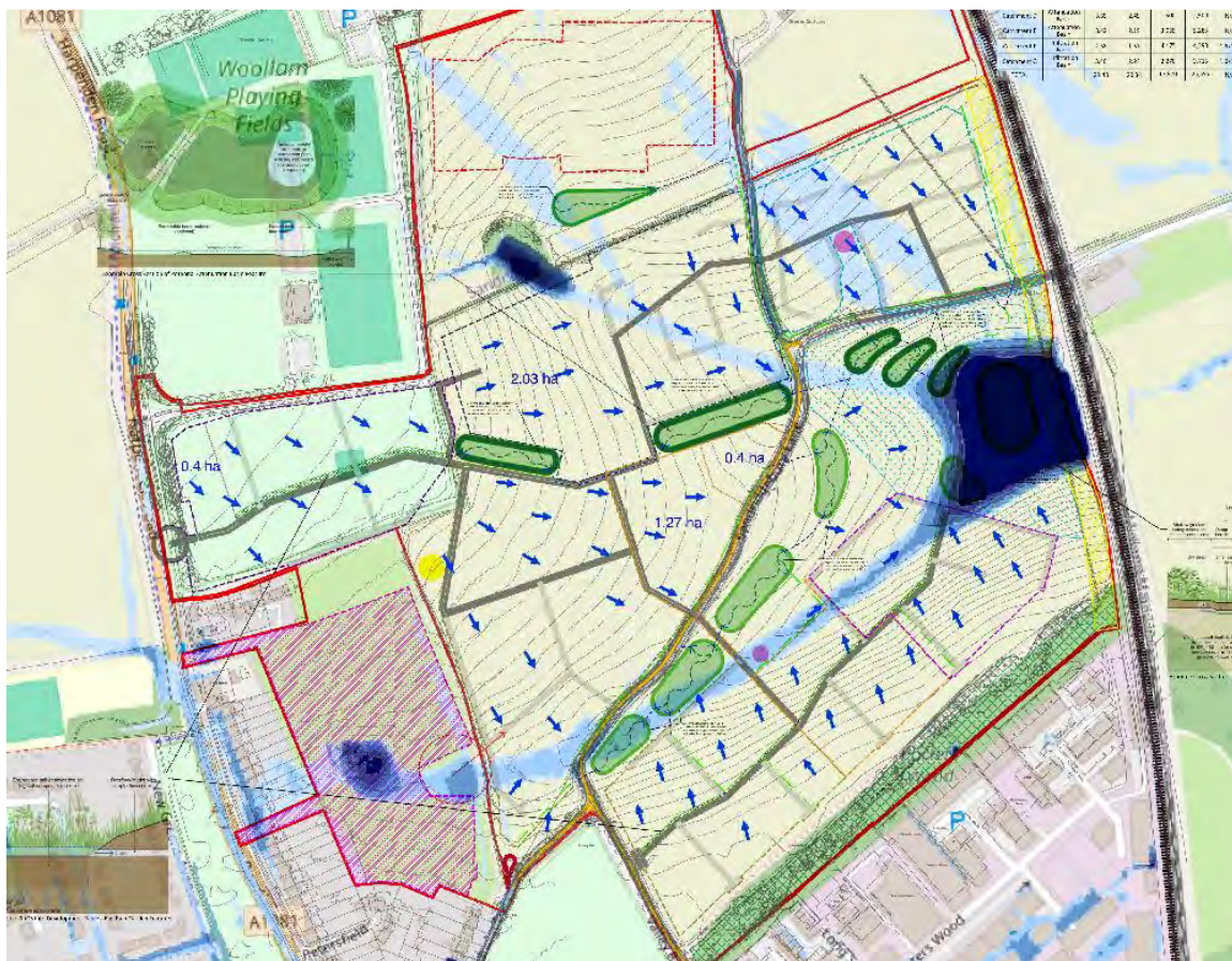
Figure 1: Overlay of the development preliminary surface water drainage strategy (May 2024) and the long term risk from surface water flooding (Environment Agency).
