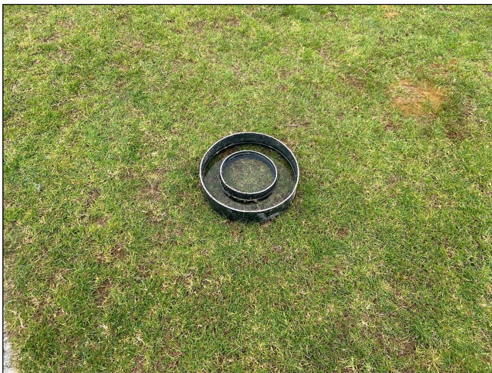
Figure 17 Example of infiltration testing using a double ringed infiltrometer (OA's Pitch 4)
