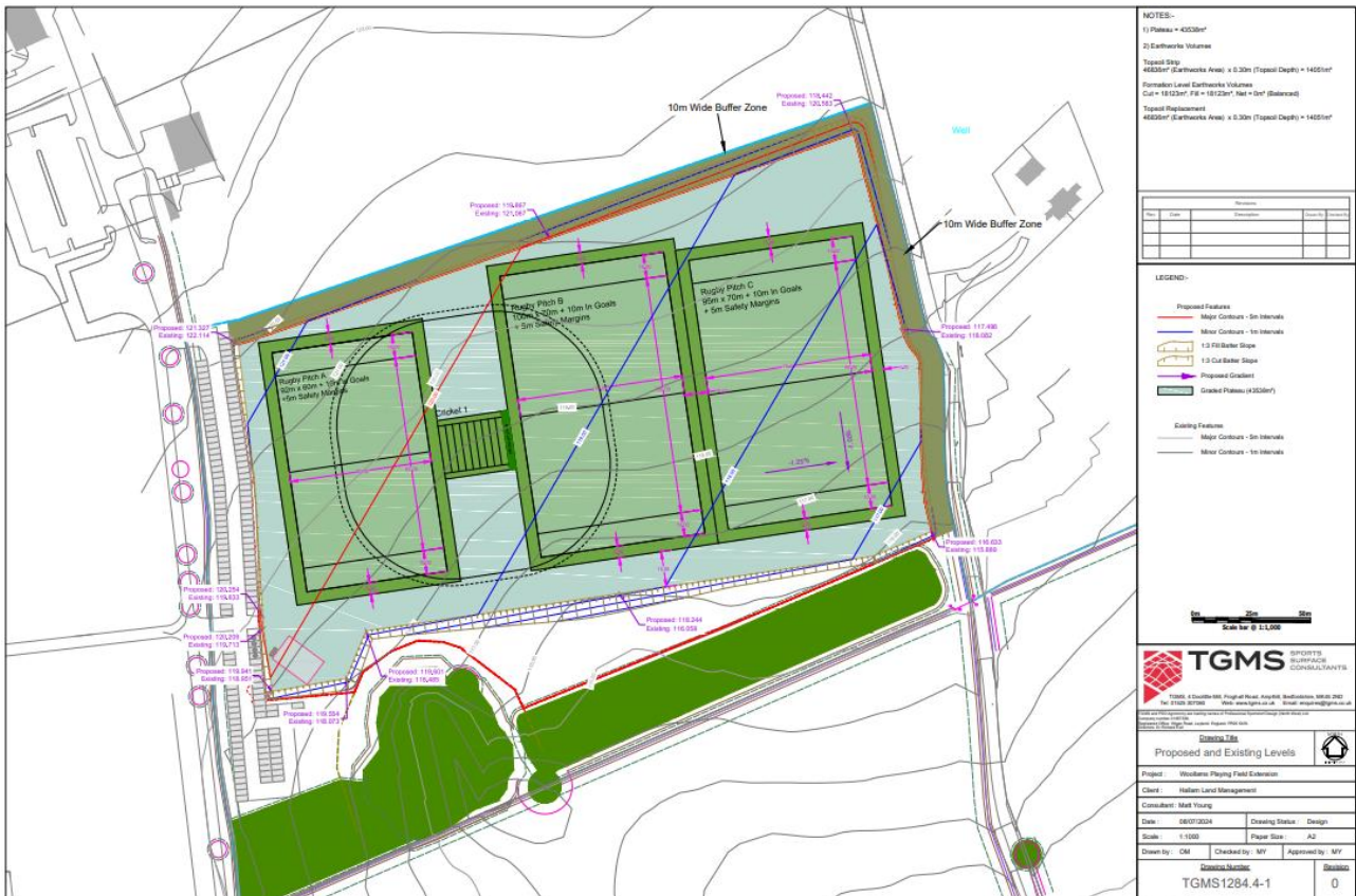
Figure 14 Proposed indicative layout by TGMS providing 3 Nr. replacement rugby pitches and a 9-pitch cricket square plus non-turf match pitch
