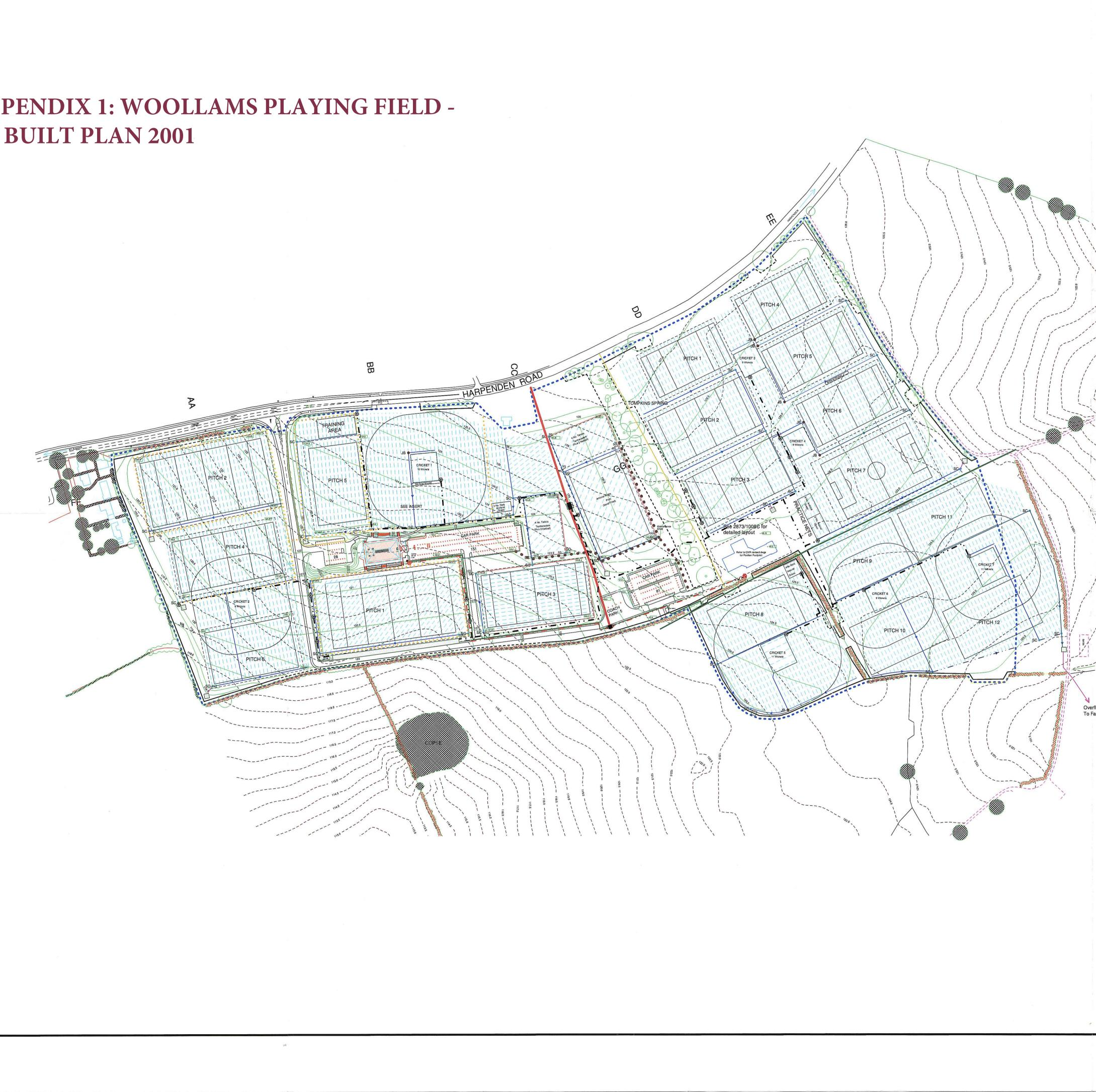
NOTES 1.) All lateral drains shown at 4m spacing on natural turf playing areas. 2.) All lateral drains on tennis courts and all-weather pitch shown at 6m spacing. 3.) - - - - - Suggested alteration to proposed contour on St Albans pitch No.2. IT IS THE CONTRACTORS RESPONSIBILITY TO ASCERTAIN THE LOCATION OF ALL SERVICES PRIOR TO COMMENCEMENT OF WORK. SETTING OUT SHALL BE THE RESPONSIBILITY OF THE CONTRACTOR, ANY DISCREPANCIES SHALL BE REPORTED AND CLARIFIED AT THE EARLIEST OPPORTUNITY.
