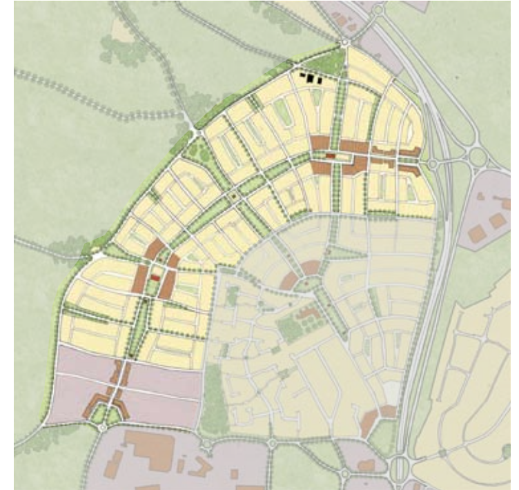
A more substantial urban extension continues with the urban pattern established by the first extension, creating a continuous thoroughfare and a linear park. Two retail centres anchor the two urban villages with pedestrian sheds of five-minute's walk.
