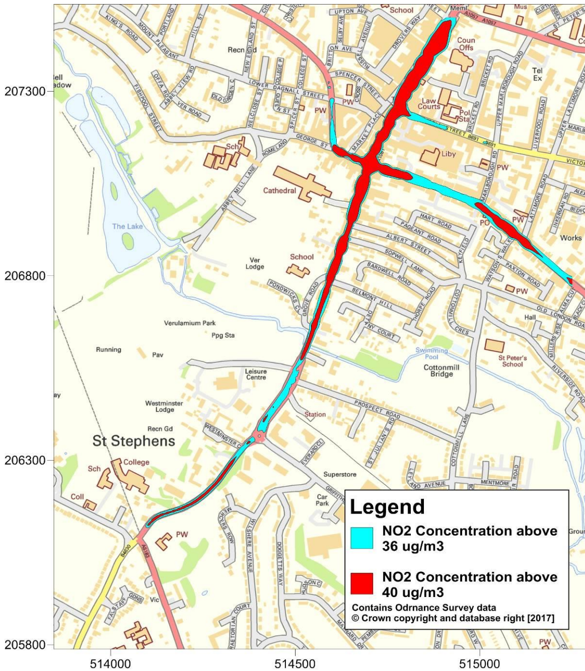
Figure A4 - Annual Mean NO 2 concentration isopleths for the V2 BC scenario (µg/m 3 )
