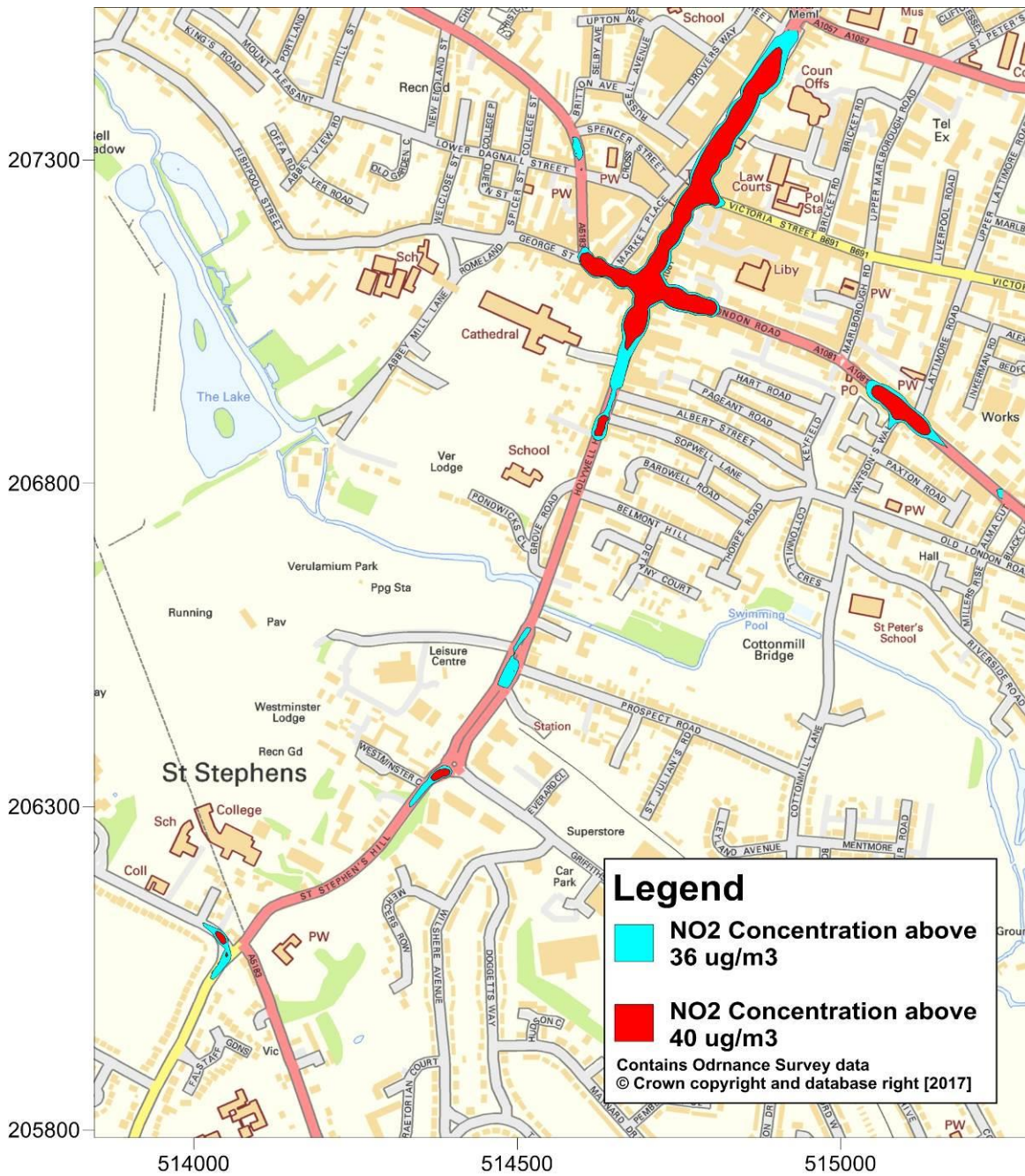
Figure A8 - Annual Mean NO 2 concentration isopleths for the V3 GC scenario (µg/m 3 )
