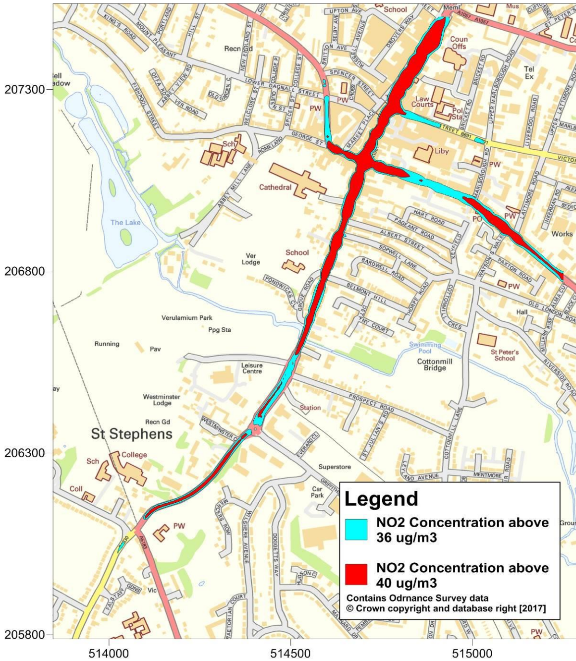
Figure A1 - Annual Mean NO 2 concentration isopleths for the V1 BC scenario (µg/m 3 )
