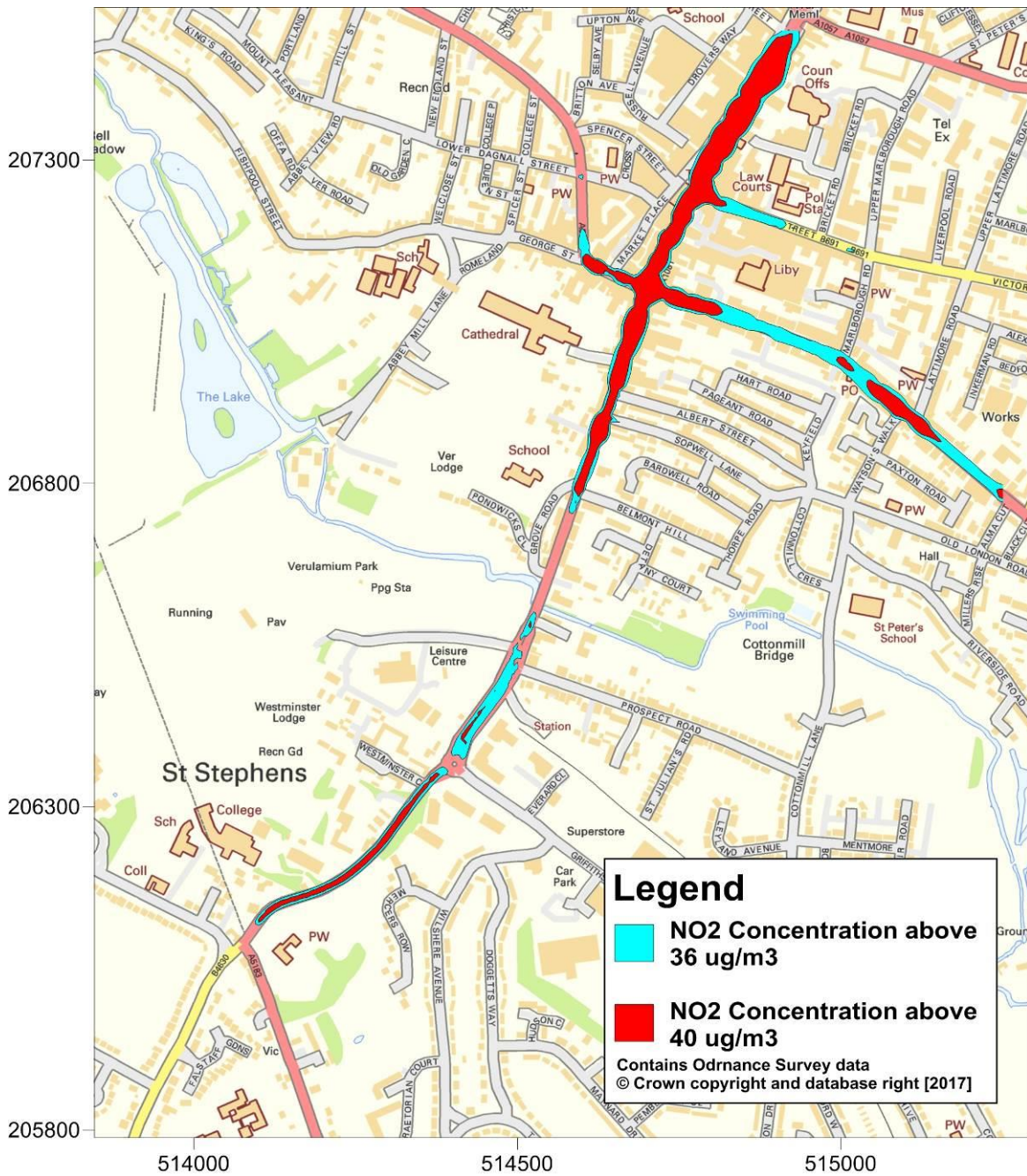
Figure A5 - Annual Mean NO 2 concentration isopleths for the V2 GC scenario ( \mu\text{g}/\text{m}^3 )
